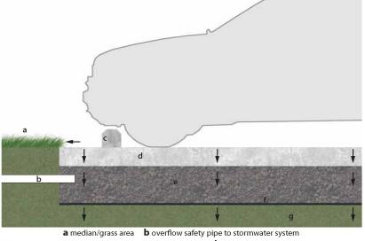
C concrete wheel stop or curb with curb gaps d pervious concrete or asphalt
